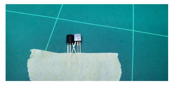
As shown there is a little ledge you can rest the soldering iron tip against to warm the legs and then dab with a small bit of solder.
