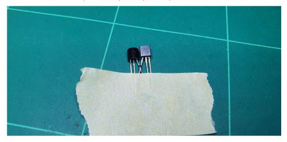
Finally, carefully cut off one of the legs at the join and bend the remaining leg straight.
