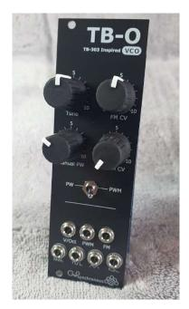
Due to the way the TB-303 wave-shapes the saw into the square, when adjusting the PW it changes both the offset and the amplitude of the waveform. Be careful at extreme PW settings both via the knob and CV control as the signal can get quite hot – extending outside the normal 10V p2p of Eurorack.
