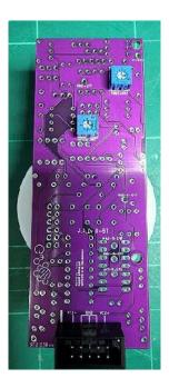
9. Finally, the headers to join the two boards. (Pictures in this section for example only, not actual production level PCBs)
