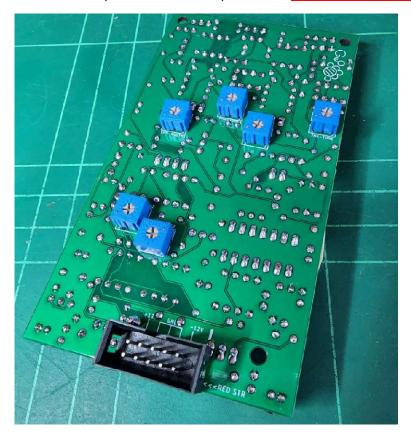
9. Finally, the headers to join the two boards.
