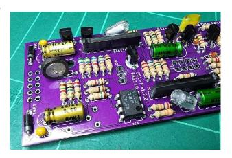
10. Add the Euro 10pin header and the 3pin trimmers on the reverse side of the board.
