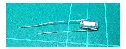
Note around C6 that the space is tight and be sure not to have the styrene leg short against the end of the electrolytic. Here I usually insert opposite to the silkscreen.
