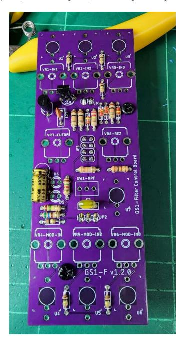
Insert **but do not solder yet** the pots, toggle switch and the jack sockets. Add the LED and place the front panel over them so you can ensure they line up with the holes.
