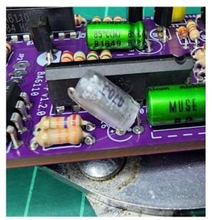
The last part on the top here is the NTC, bend the legs gently apart so that it will go into the holes easily and sit more or les flush with the PCB.
