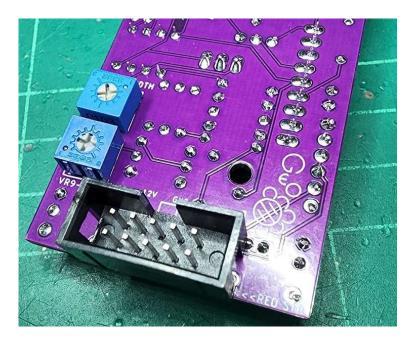
11. Finally, the headers to join the two boards.
