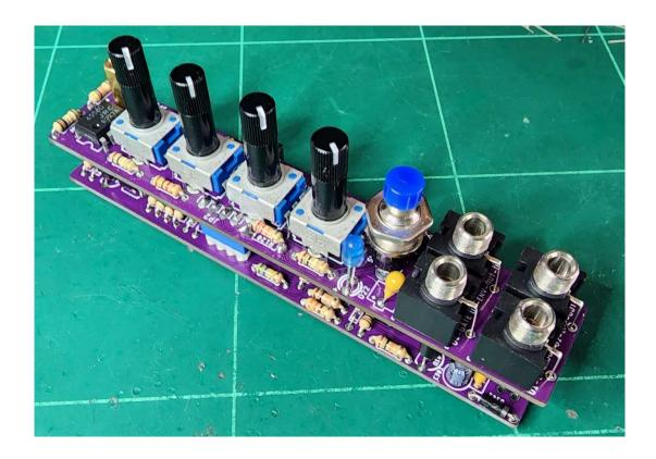
Insert **but do not solder yet** the pots, switch and the jack sockets. Add the LED and place the front panel over them so you can ensure they line up with the holes.
