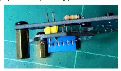
3. When you are happy that its all lining up, push the two board together as close and parallel as you can so the plastic on the pin strip is even all around then solder the rest of the pins on the underside. Push down slightly as you solder so it stays flush.
