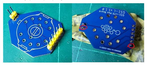
2. Insert the mez board into the upper board as shown. You may need to heat and adjust one of the pins you soldered if they are not lining up.
