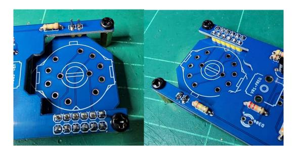
Before we insert the rotary switch check all the pins are straight and bend the locator tab flat as shown and insert it carefully into the mez board **but do not solder yet.**
