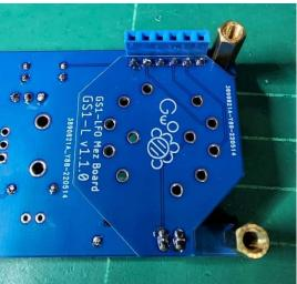
4. Now repeat the process on the top side, solder just one pin on each strip, check its all flush and then solder them all. Finally trim the excess pins.
