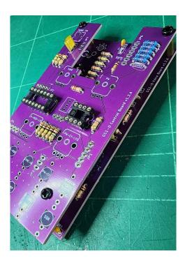
8. Once done I like to clean the flux off the voice board at this point then finally, add the Euro 10pin header and the 3pin trimmers on the reverse side of the board.
