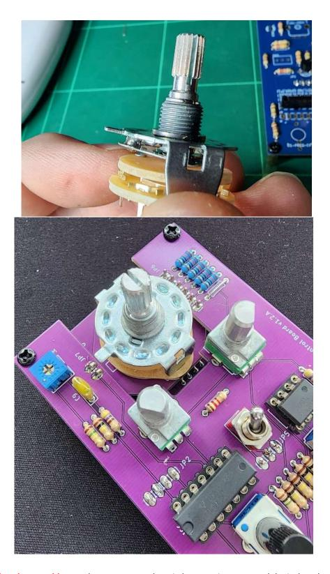
Insert **but do not solder yet** the pot, two toggle switch, potentiometers and the jack sockets.
