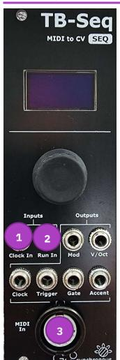
Clock In - A CV input jack that receives a pulse on a regular interval. The number of pulses that are received before the sequencer moves on to the next step is determined by the CV Clock In – PPQN setting.
