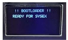
To exit bootloader mode without sending an update press the reset switch on the side of the module, or power cycle the module.
