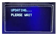
When the download is complete, assuming it was successful, the device will briefly show the message below and will automatically reboot. You should see that it is now running the new version in the boot splash screen.
