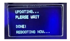
If the device doesn't reboot, or you don't see the BOOT LED flashing, check your MIDI configuration in your SysEx tool. Sometimes you may need to either reduce the SysEx tool buffer size and/or add a delay between each buffer in your SysEx tool.
