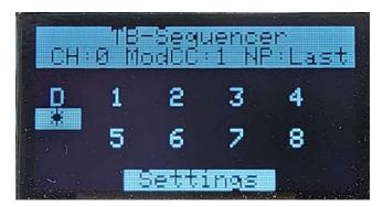
When the device is ready for use it will show the "home page". This shows some basic MIDI configuration details in the header, a list of the slots showing which ones have sequences stored and which is the currently activated sequence.
