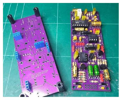
3. Finally add the pots and jack sockets and use the panel to line then up correctly before soldering.
